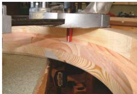
▲ Pic.11 Mark the frame position, remove and mount upside down. Rout the rebate for the glass
